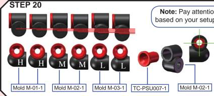
**Note:** Pay attention to the orientation of the suspension mount inserts based on your setup. The screw hole is vertically offset by 0.25mm.
